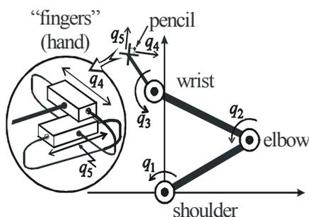
**Figure 1.** Mechanism configuration with five DOF
