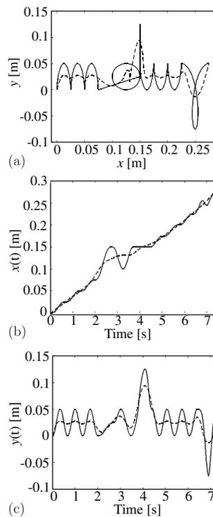
Fig. 3. Definition of the task: (a) sequence of letters; (b), (c) time histories of operational coordinates. The solid lines show the prescribed motion, and the dashed lines show the smooth components.
