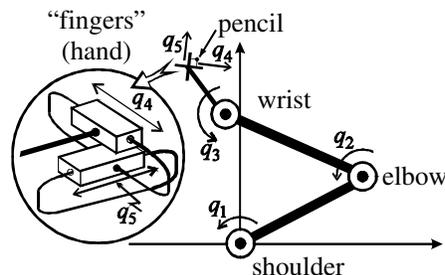
Fig. 1. Mechanism configuration with five DOF.
