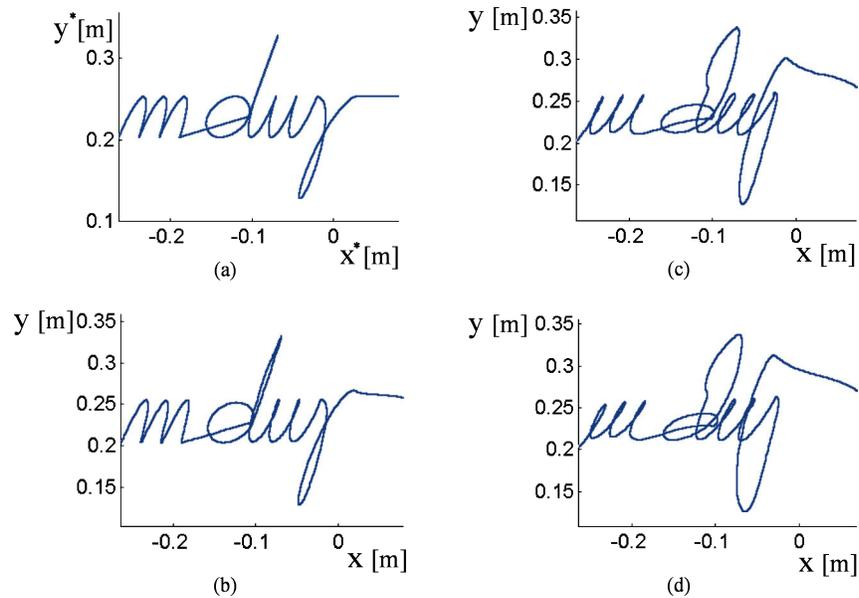
Fig. 10. Gradual degeneration of writing. (a) Reference sequence. Degenerated sequences are recorded for the following repetitions: (b) 12th forward sequence, time:  $198 \leq t \leq 207$ , (c) 14th forward sequence, time:  $234 \leq t \leq 243$ , (d) 22nd forward sequence, time:  $378 \leq t \leq 387$ .
